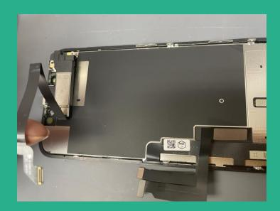
Step 20 ~ Screen, LCD, and Digitizer is removed from the frame
