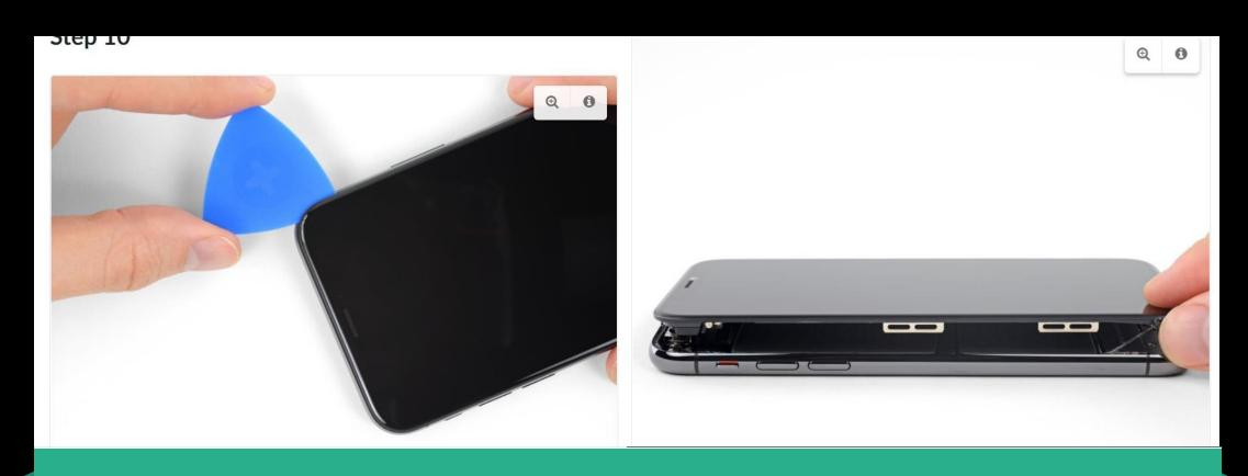
\*Pry around the edges until the screen is separated, then slowly lift
