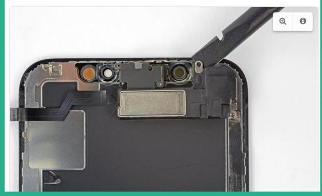
We are now removing the earpiece, microphone and the proximity sensor so that it can be transferred to the NEW screen
